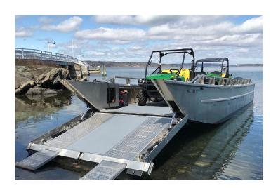
The LC19 with the <u>Maxgate</u> landing door and heavy duty hydraulics not only allows you to drive large vehicles on and off the beach, it will easily lift a truck as well.
